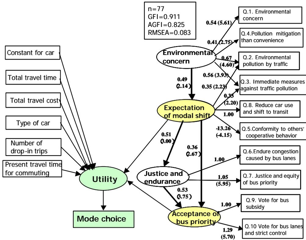
Figure 4. Integrated choice and latent variable model, Niigata.
