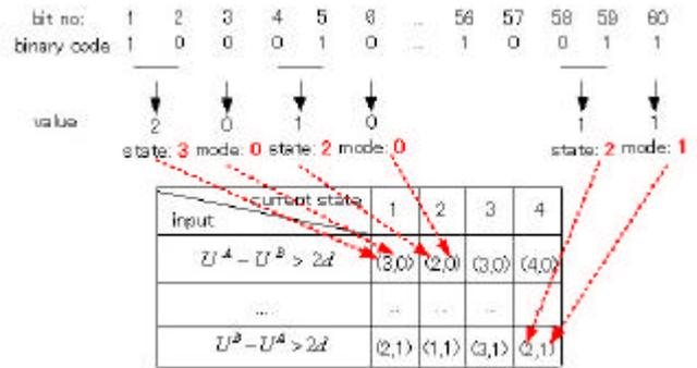
Figure 3: Decoding process of a chromosome into an FSM
