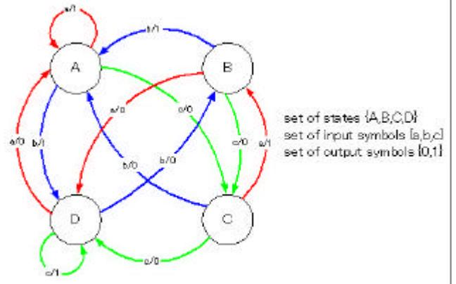
Figure 2: An illustration of an FSM
