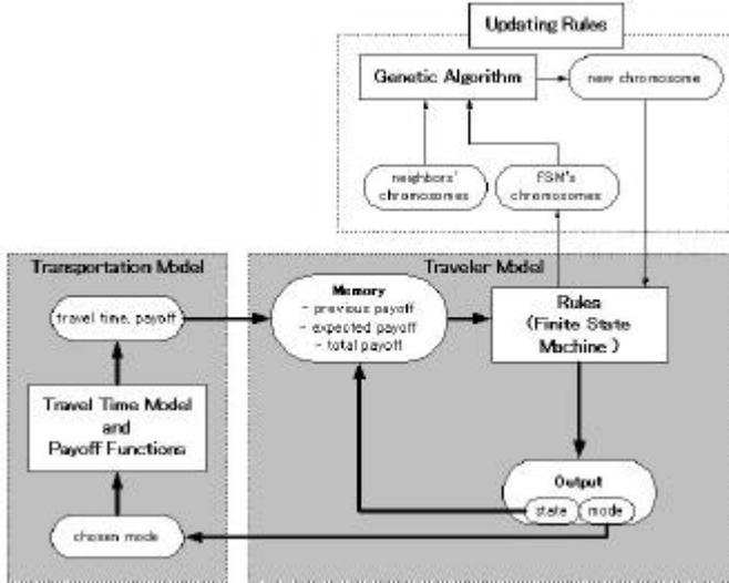
Figure 1: Multiagent simulation model utilized in order to acquire adaptive behavior.
